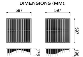
NB: Contour is made up of two differently configured tiles (Type A and Type B) to form one 1194mm x 597mm Contour tile as depicted in the photos.
