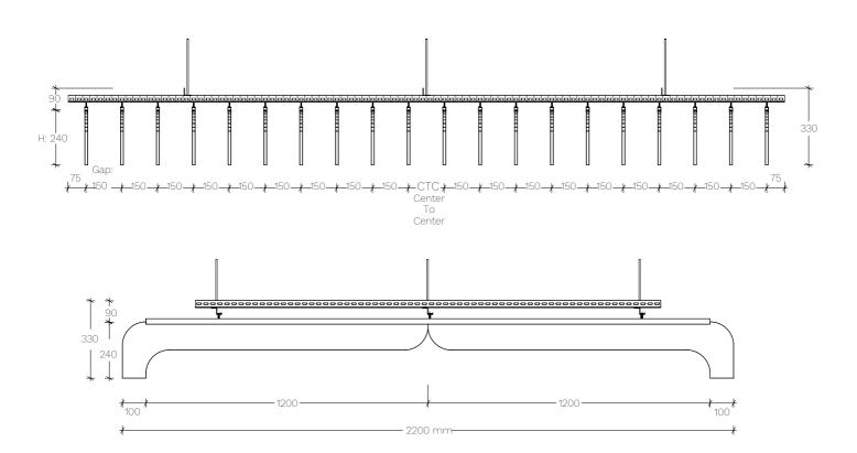
Baffle models of Plativity Collection are simple, elegant and one of the most dynamic modular acoustic ceiling systems. Easy to install, lightweight, and can be installed quickly to transform large volumes into linear ceiling systems. Baffle delivers tailor made acoustic solutions with cut-out 12mm thickness of Plate sheets that offers an adjustable gap between felt baffles and various dimensions. Upon request, we can manufacture with various thicknesses and customizable designs.
